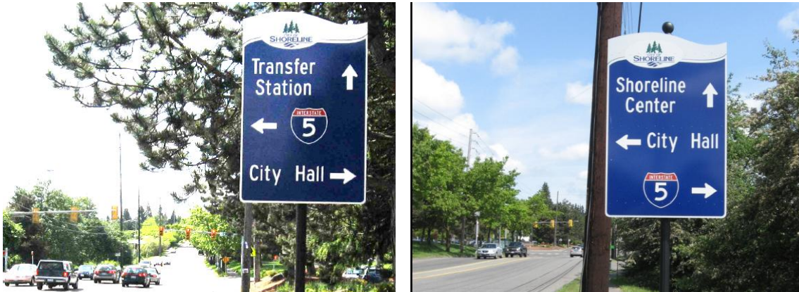
Fig 11. Wayfinding signs can be located in medians, behind sidewalks, or on poles
