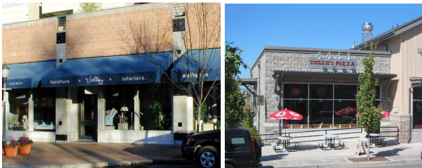
The left image uses smooth gray blocks on the vertical columns and beige split-faced blocks above the awnings. The storefront in the right image uses gray split face and some lighter, square, smooth-faced blocks below the storefront windows.
