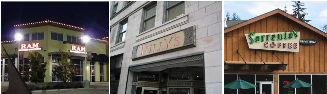
Figure 20.92.240. Permitted sign illumination techniques including individual backlit letters (left image), opaque signs where only the light shines through the letters (center image), and neon signs (right image).
