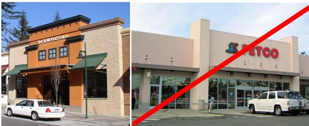
Figure 20.92.200(D). Acceptable (left) and unacceptable (right) use of synthetic stucco. The left image employs concrete near the ground level and a variety of other surface materials on the façade. The right image uses synthetic stucco for more than 50 percent of the façade and some surfaces extend to the ground level.
